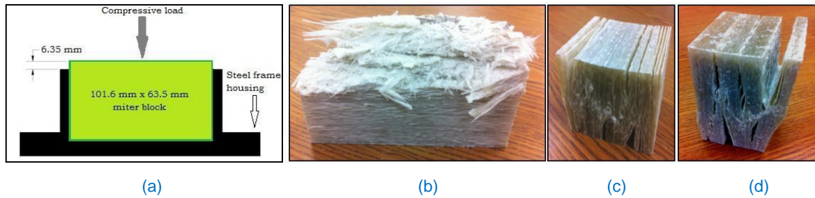
Figure 5: (a) Compression testing, failure in (b) through-thickness, (c) widthwise, (d) lengthwise
