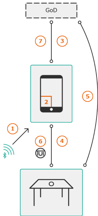
Figure 4: Shows the interaction of an active exhibit. (1) OD recognizes the table's Bluetooth beacon, (2) OD identifies the table with the lookup table, (3) OD registers new location at GoD ( atExhibit ) and receives the table's content package, (4) OD opens connection to the table, (5) table requests the OD's information (e.g., IP address), (6) table communicates with the OD by means of TUIO, (7) OD registers onExhibit at GoD.
