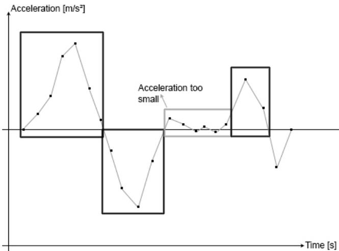
Fig. 3. Peak detection and minimum threshold (along z-axis).
